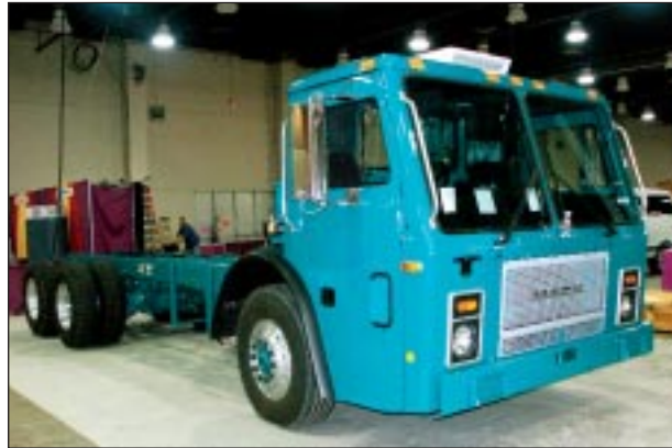
Mack truck chassis here has an E7G-325 engine fueled by LNG.
